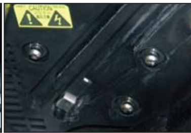
21. HV contact inside a LJ 4100, second from right; Round HV contacts in an 8150, right. The metal clip is a ground.
