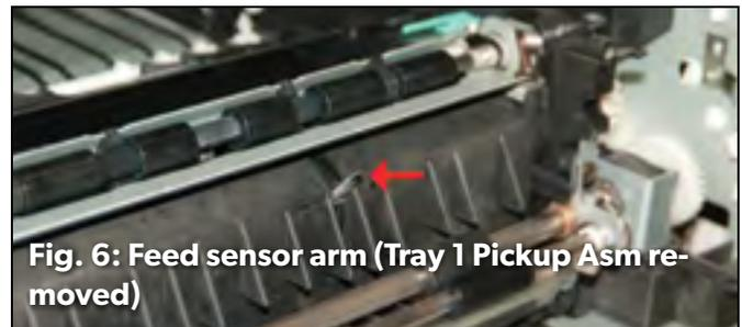
**Fig. 6: Feed sensor arm (Tray 1 Pickup Asm removed)**
