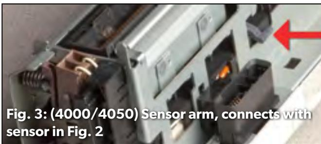
**Fig. 3: (4000/4050) Sensor arm, connects with sensor in Fig. 2**
