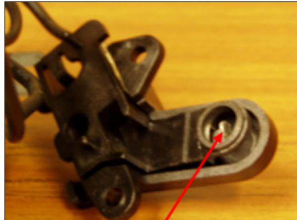
Figure 2: Inner side of end cap, showing metal contact strip (red arrow)
