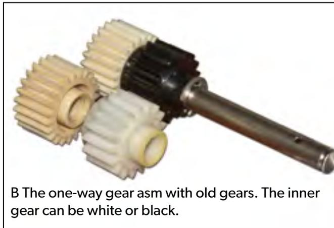
B The one-way gear asm with old gears. The inner gear can be white or black.
