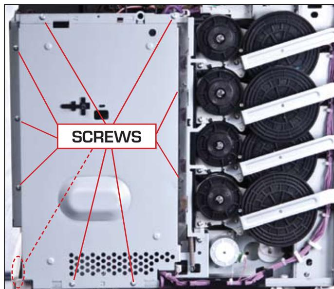
**9** DC Controller Shield Removal
