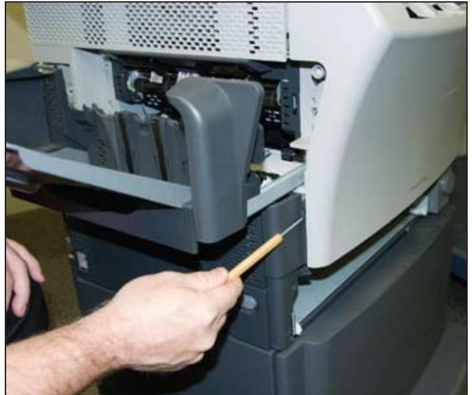
G. Release the retaining tab on the left side of the front cover. This one seems prone to breaking.
