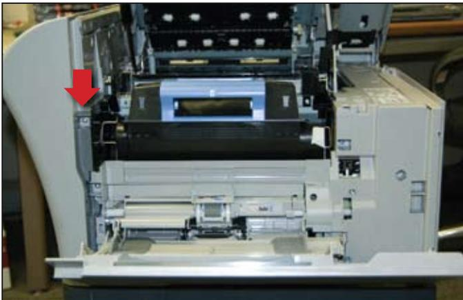
D. Open the top cover and remove one screw.
