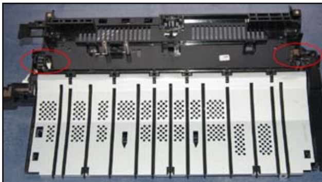
Fig. 1 Feeder Assy without transfer roller, connection points circled.
