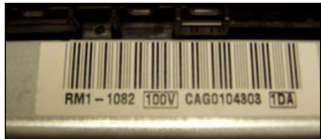
Figure 2: Part Number Label on 4240/4250/4350 Fuser (RM1-1082)
