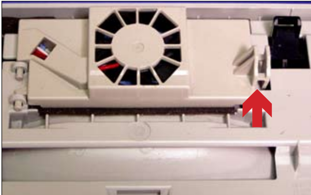
Figure 4: Fan door and retaining clip (squeeze and pull to open door)
