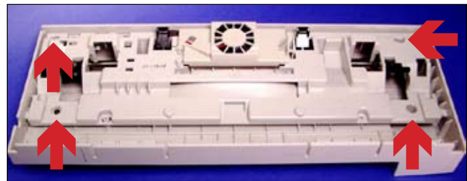
Figure 2 (arrows show 4 screws to remove)
