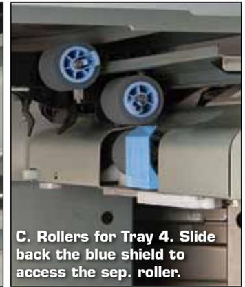
C. Rollers for Tray 4. Slide back the blue shield to access the sep. roller.
