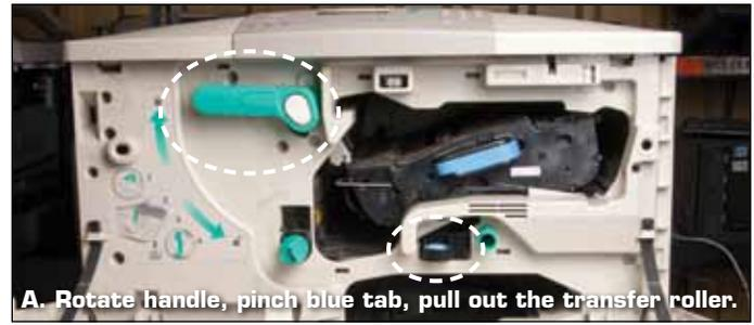
A. Rotate handle, pinch blue tab, pull out the transfer roller.
