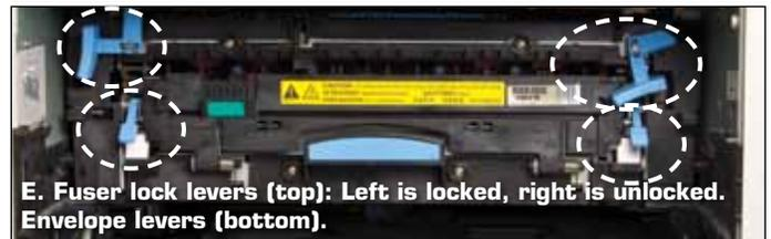
E. Fuser lock levers (top): Left is locked, right is unlocked. Envelope levers (bottom).
