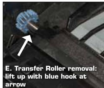
**E. Transfer Roller removal: lift up with blue hook at arrow**
